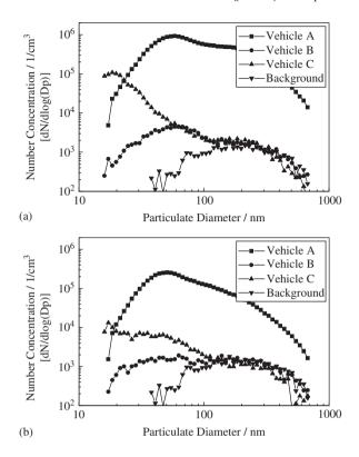
Fig. 6. Size distributions of particulate for different vehicles. (a)  $x = 0.5 \,\mathrm{m}$ ,  $y = 0.0 \,\mathrm{m}$ , and  $z = 0.0 \,\mathrm{m}$ ; (b)  $x = 1.0 \,\mathrm{m}$ ,  $y = 0.0 \,\mathrm{m}$  and  $z = 0.0 \,\mathrm{m}$ .
