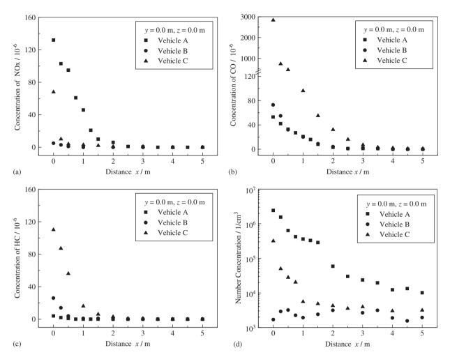
Fig. 5. Comparison of NO<sub>x</sub>, CO, HC and particulate number concentration in exhaust flume of different vehicles.
