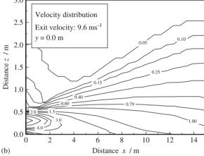
Fig. 12. Distribution of flow velocity under different exit velocities.
