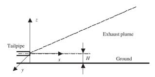
Fig. 1. Schematic of the Cartesian coordinate system and vehicular exhaust plume geometry.
