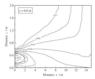
Fig. 9. Distribution of CO relative concentration under different initial CO emission concentration (exit velocity: 4.8 m s<sup>-1</sup>).
