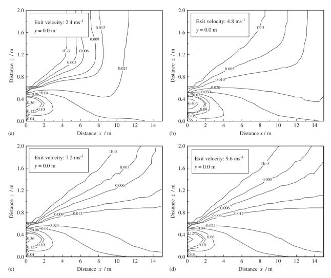
Fig. 11. Distribution of CO relative concentration under different exit velocities.
