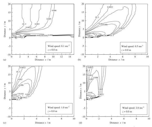
Fig. 14. Distribution of CO relative concentration under different crosswind speeds (exit velocity: 4.8 m s<sup>-1</sup>).
