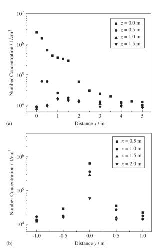
Fig. 3. Particulate number concentration at different sampling points for vehicle A. (a)  $y = 0.0 \,\mathrm{m}$ ; (b)  $z = 0.0 \,\mathrm{m}$ .
