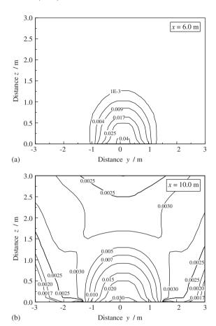
Fig. 10. Distribution of CO relative concentration in the section y-z for downstream distances of 6 and 10 m (exit velocity:  $4.8 \text{ m s}^{-1}$ ).
