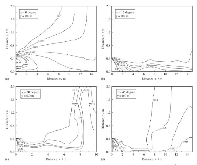
Fig. 13. Distribution of CO relative concentration under different tailpipe exit direction (exit velocity: 4.8 m s<sup>-1</sup>).
