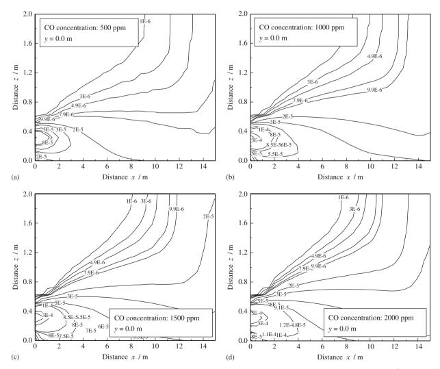
Fig. 8. Distribution of CO concentration under different initial CO emission concentration (exit velocity: 4.8 m s<sup>-1</sup>).
