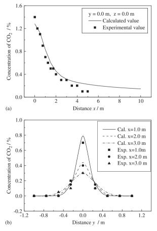
Fig. 7. Comparison of  $CO_2$  concentration between the experimental data and simulated results. (a)  $y = 0.0 \,\mathrm{m}$ ; (b)  $z = 0.0 \,\mathrm{m}$ .
