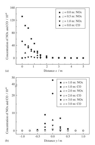
Fig. 2. Concentrations of  $NO_x$  and CO at different sampling points for vehicle A. (a)  $y=0.0\,\mathrm{m}$ ; (b)  $z=0.0\,\mathrm{m}$ .
