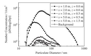
Fig. 4. Size distributions of particulate at different locations for vehicle A.
